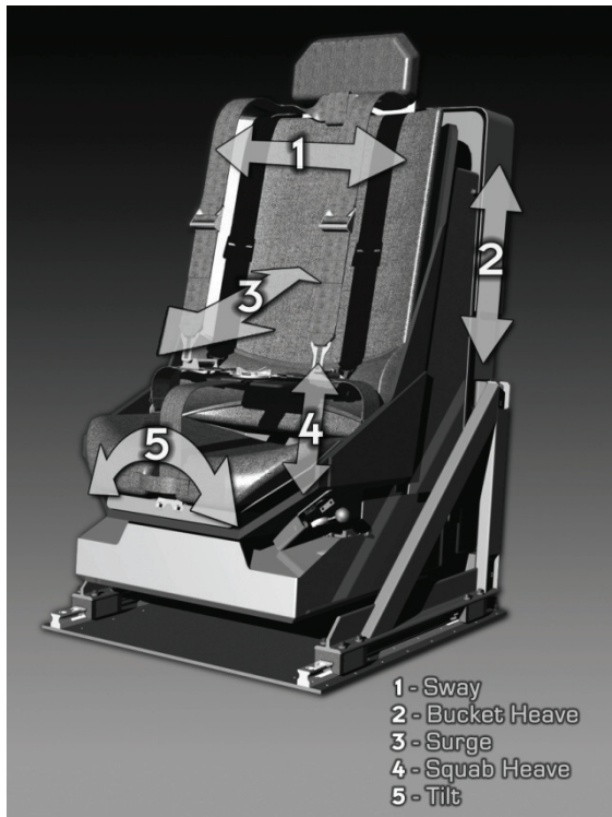
Figure 1 Direction of Movement in a Five-Axis Dynamic Motion Seat
