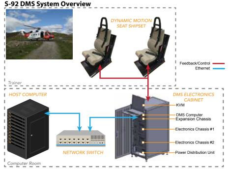
Complete S-92 Dynamic Motion Seat System includes the seats, computer, electronics, and cables to drive the seats.
