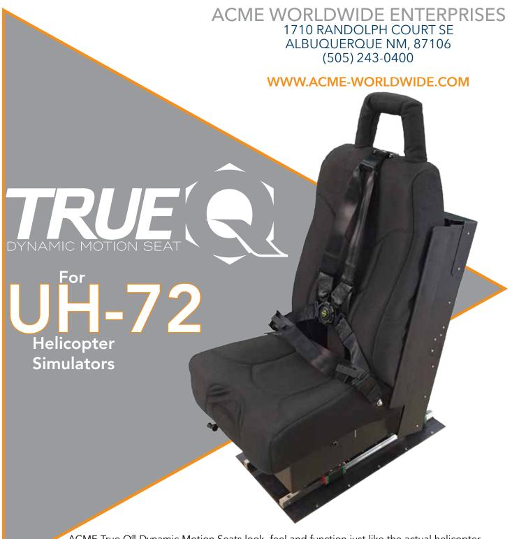
ACME True  $Q^{\otimes}$  Dynamic Motion Seats look, feel and function just like the actual helicopter seats. All the motion components are inside the seat. The seats translate simulator acceleration signals into realistic, convincing motion cues that emulate the forces and sensations felt in flight.
