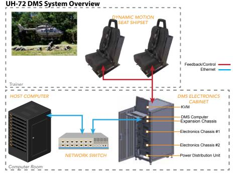
Complete UH-72 Dynamic Motion Seat System includes the seats, computer, electronics, and cables to drive the seats.
