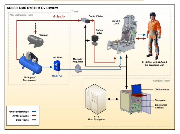
Complete system includes all the components needed to translate acceleration signals from the flight model into realistic motion cueing. System includes executable software to drive the seat system. One computer can drive it all: The motion seat computer can support two seats using the same flight model (Pilot/Co-Pilot) and the Optional G-Suit and Mask Air systems.
