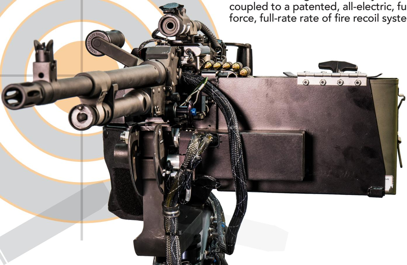
A full set of sensors monitor the weapon status and gunner's actions. Replaceable ammo cans and reloading logic train gunners to load, feed, charge, and fire quickly and correctly.
